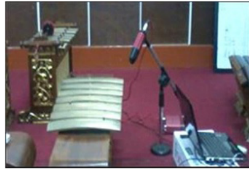
Figure 1. The arrangement of instrument to extract the acoustic data from the OD.
